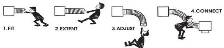
The **STRETCHDEC** fulfills all the requirements and are classified as specified within EN 13180: *Ventilation for buildings – Ductwork - Dimensions and mechanical requirements for flexible ducts.*
