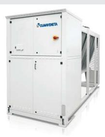
Outdoor unit for the production of chilled water with fixed speed and variable speed (Inverter Driven) Scroll compressors, optimized for R410A in a single-circuit configuration, axial-flow fans, micro-channel full-alluminum air coils and electronic expansion valve as standard equipment.
