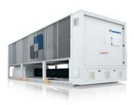
Outdoor unit for the production of chilled water with fixed speed and variable speed (Inverter Driven) screw compressors optimized for R134a, axial-flow fans, condensing coil with copper tubes and aluminium fins, shell and tube single pass evaporator designed by Climaveneta and electronic expansion valve.
