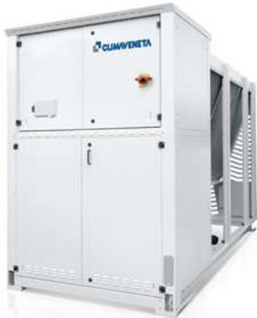
Multi-purpose outdoor unit for use in 4-pipe systems for the simultaneous production of chilled and hot water by means of two independent hydronic circuits. These units are able to satisfy the demand for hot and cold water simultaneously through a system that does not require seasonal switching and is therefore a valid alternative to traditional plants with chiller and boiler.
