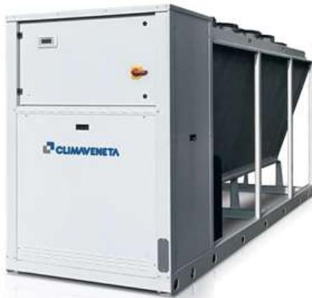
Outdoor unit with heat pump for the production of chilled/hot water with hermetic rotary scroll compressors dedicated to the use of R410A, axial fans, plate heat exchanger, condensing coil with copper tubes and aluminum fins and thermostatic or electronic expansion valve, according to the version. The range is composed by units equipped with two compressors in a single-circuit configuration.
