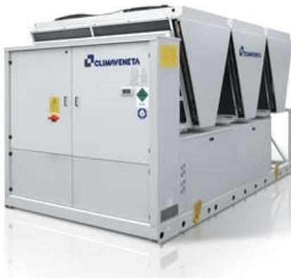
Outdoor heat pump for the production of chilled/hot water with hermetic rotary Scroll compressors, ozone-friendly refrigerant R410A, axial-flow fans, shell and tubes exchanger and electronic expansion valve. The range is composed by units equipped with four, six and eight compressors in multi-circuit configuration.
