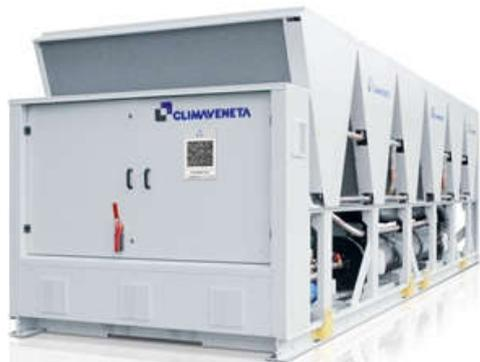
Outdoor unit for the production of chilled water with semi-hermetic screw compressors optimized for HFO refrigerant R1234ze, axial-flow fans, micro-channel full-aluminum condensing coils, single-pass shell and tubes evaporator designed by Mitsubishi Electric Hydraulics & IT Cooling Systems S.p.A. and electronic expansion valve.
