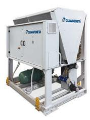
Outdoor unit for the production of chilled water with semi-hermetic screw compressor optimized for R134a, axial-flow fans, micro-channel full-aluminum condensing coils, single-pass shell and tubes evaporator designed by Mitsubishi Electric Hydronics & IT Cooling Systems S.p.A. (brazed plate evaporator for sizes 0751 and 0851) and electronic expansion valve.
