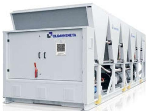
Outdoor unit for the production of chilled water with semi-hermetic screw compressors optimized for R134a, axial-flow fans, micro-channel full-aluminum condensing coils, single-pass shell and tubes evaporator designed by Mitsubishi Electric Hydronics & IT Cooling Systems S.p.A. and electronic expansion valve.
