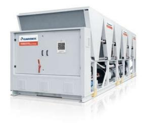
Outdoor unit for the production of chilled water with semi-hermetic screw compressor optimized for R513A, axial-flow fans, micro-channel full-aluminum condensing coils, single-pass shell and tubes evaporator designed by Mitsubishi Electric Hydronics & IT Cooling Systems S.p.A. (brazed plate evaporator for sizes 0751 and 0851) and electronic expansion valve. Base and supporting structure and panels are of galvanized epoxy powder coated steel with increased thickness. Eurovent certification.
